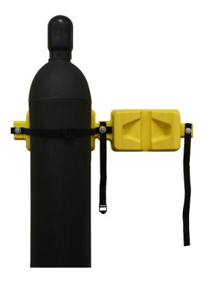
This simple, yet effect bracket immediately improves workplace safety by providing secure storage for any number of cylinders from 3"-10" in diameter. The plastic design is lightweight, durable, and non-sparking. The unique design allows an unlimited number of brackets to be strung together. Great for cylinder storage or transport.
